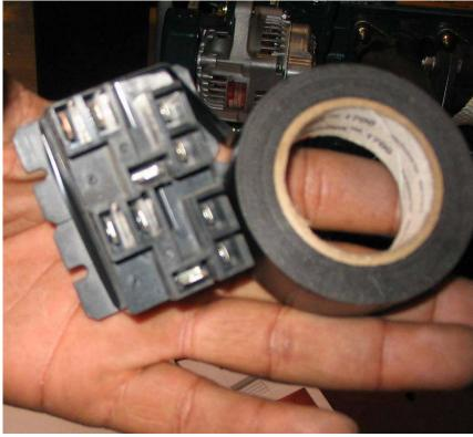
Wrap electrical tape around both RELAYS-12 VDC SPDT so they are bound together and look like one relay.
